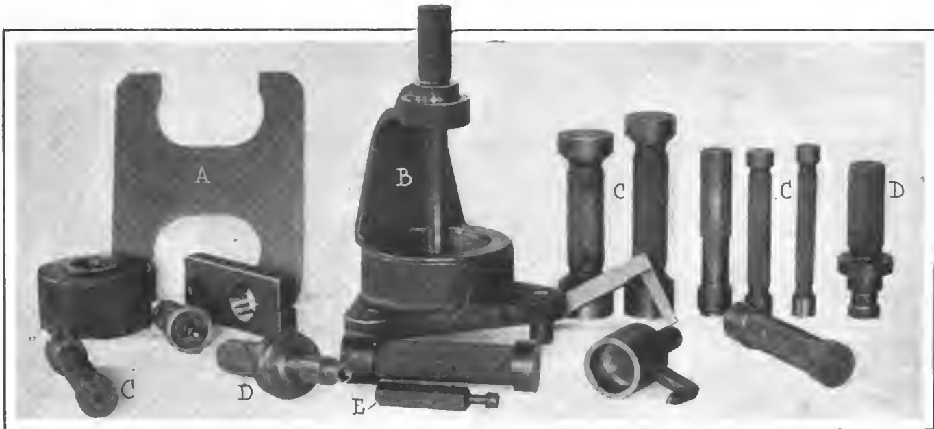
An array of gauges for testing various dimensions of the Holley carburetor to a thousandth of an inch. Most of these work on the "Go" and "No Go" principle. A—External diameter or width gauge. B—Distance gauge. C—Plug gauges for internal diameters. D—Depth gauges. E—Thread gauges. The rest are special gauges for testing certain parts.
